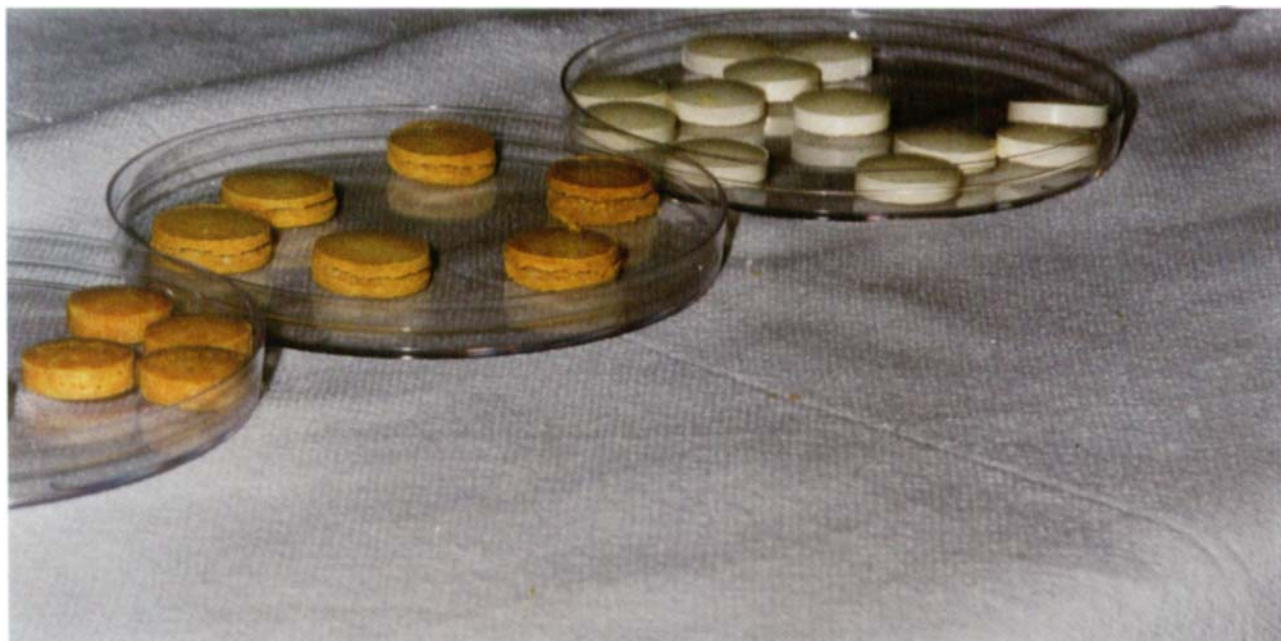
Figure 12. Effect of high humidity on tablets containing amoxicillin and clavulanic acid. Orange color is associated with clavulanic acid degradation. Right: triple-layer stearic acid formulation; center: Augmentin® 250 mg chewable; left: single-layer formulation containing all ingredients of triple-layer stearic tablets.
